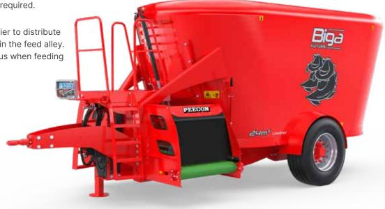
Unloading doors are optionally available with a height-adjustable conveyor belt. Some models are also available with a chain conveyor instead of a conveyor belt.
